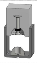
The steel recess formers SBK and SBKM are always used in combination with a rubber ring. The rubber ring ensures that the anchor fits snugly in the former. Moreover, the rubber ring prevents concrete pouring into the recess former.
