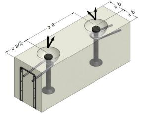
The angled pull reinforcement must be mounted opposite the direction of the load
