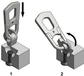
The clutch is placed in the right position.
