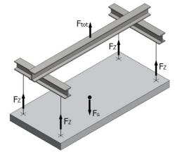
The compensating lifting slings ensure equal force distribution. Load bearing anchors: n=4
