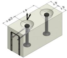
The angled pull reinforcement must be mounted opposite the direction of the load
