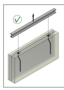
To prevent concrete spalling, we recommend using a spreader beam when precast elements must be lifted and transported or during installation.
