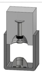
When using this magnetic recess former, it is very important that the surface of the formwork is clean. After demoulding, the magnetic former can be removed from the formwork with a screw.
