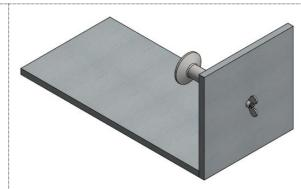
For wooden formwork, the recess former can be mounted with the OPR mounting plate. The pins on the OPR ensure that the recess former remains closed when pouring concrete. The OPR is mounted on the formwork with nails.
