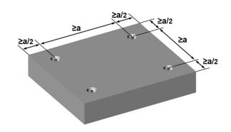
L = anchor length a/2 = edge distance e = cover to anchor head R = recess radius
