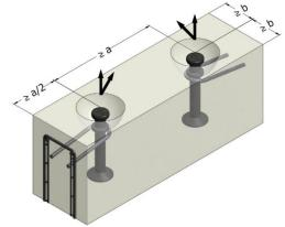
The angled pull reinforcement must be mounted opposite the direction of the load
