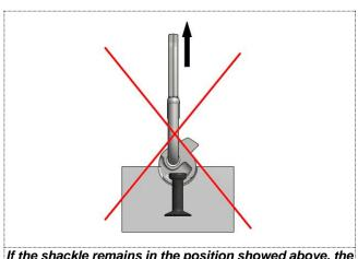
If the shackle remains in the position showed above, the lifting of the concrete unit is not allowed
