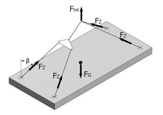
Lifting of wall elements parallel to the axis of concrete element Load bearing anchors: n=2
