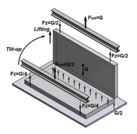
Lifting the walls from horizontal to vertical position without tiltup table.
