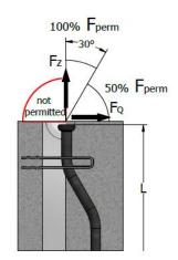
Angled pull with cable/chain spread of  $\beta > 30^{\circ}$  is not permitted
