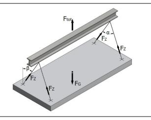
Perfect static weight distribution can be obtained using a lifting beam and two pairs of anchors symmetrically placed.
