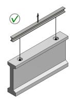
Diagonal load  $\beta = 10^{\circ}$  to 45° Note:  $\beta \leq 30^{\circ}$  is recommended
